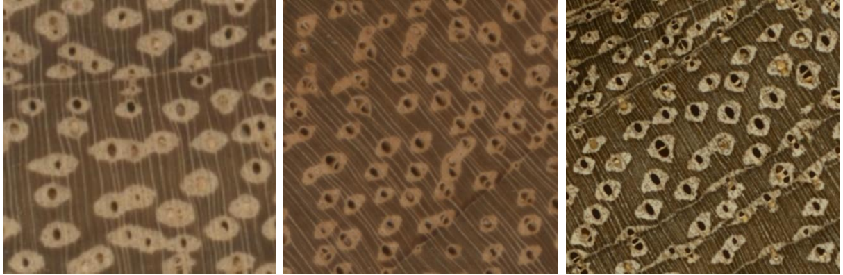
Figure 5.2: Example of hard triplet consisting of an anchor (left: Afzelia; Tw11081), positive (centre: Afzelia; Tw47200), and negative image (right: Anthonotha; Tw95) for Object Re-Identification network training with triplet loss.
