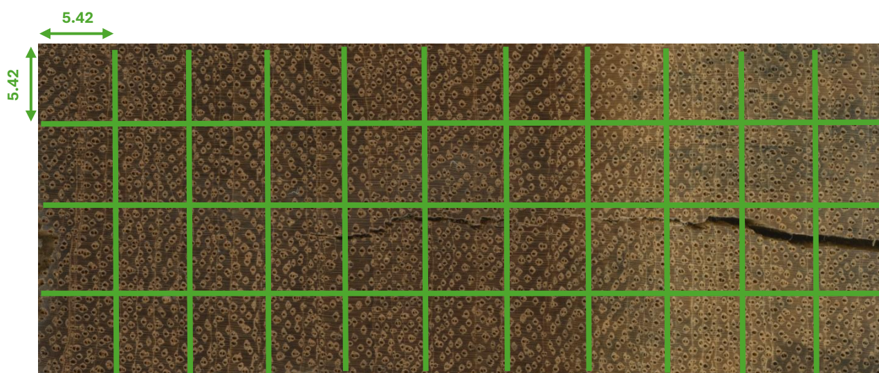
Figure 1.4: An example of a typical image in the SmartWoodID collection (Tw26431), cropped into patches of 5.42 \times 5.42 mm.
